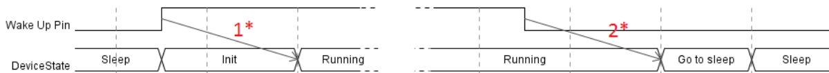
Figure 10: Timing for Low Power On, programmed to wake up on wake up pin
