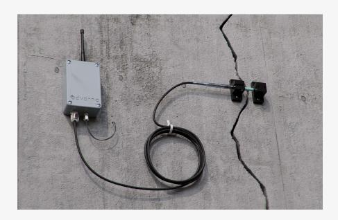
Advarna facilitates real-time crack monitoring with ATIM radio modules
