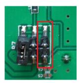
When the ARM-Nano EV is connected to a PC via a USB cable, it can draw power from the USB bus. The onboard voltage regulator supplies approximately 3.3V to the board. The power source selection jumpers should short circuit pin 3-4 ("USB") of header.
